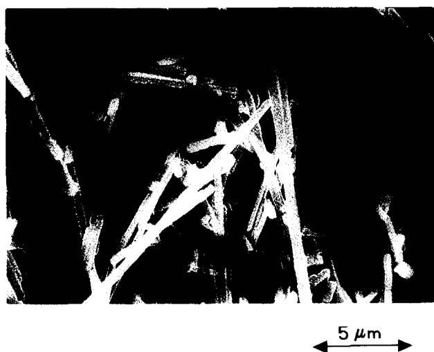
Figure 1 SEM photomicrograph of potassium titanate whiskers
